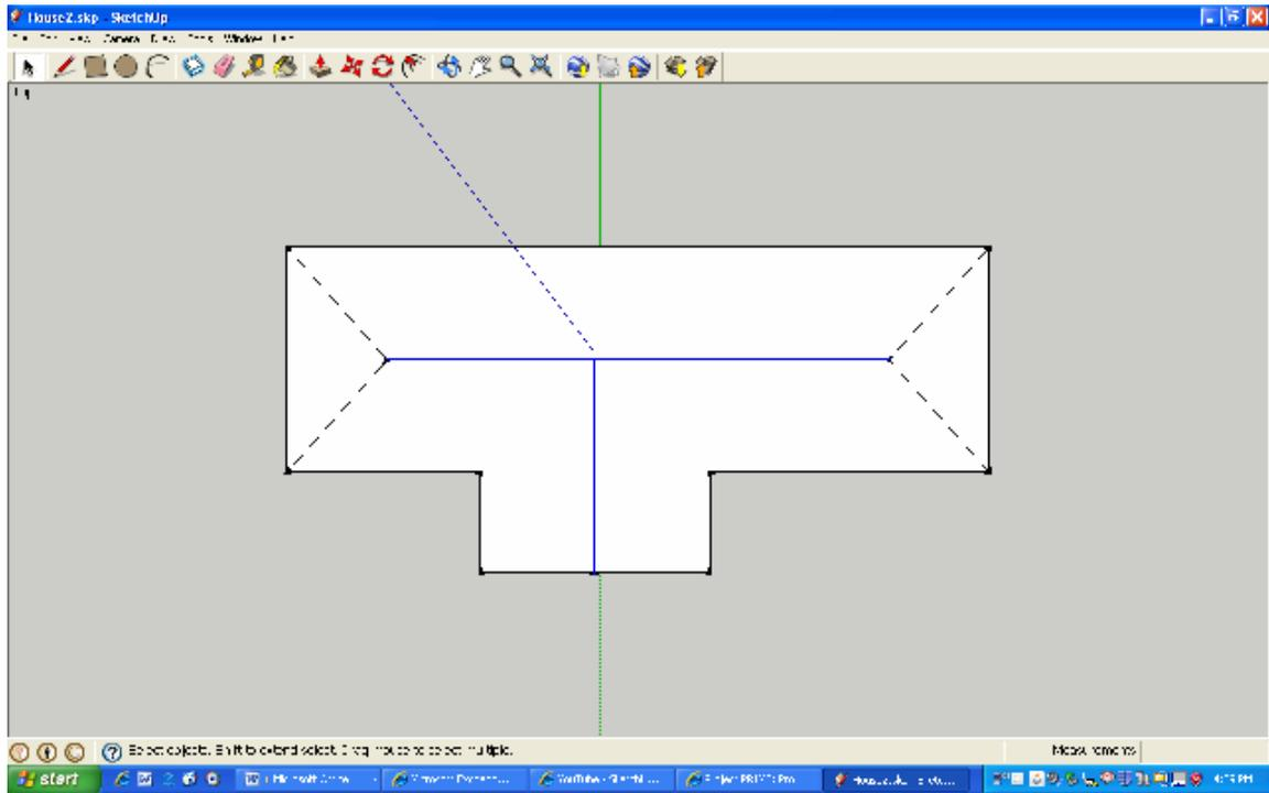
**Fig. 9** Top view of house with lines drawn in for roof hips, valleys, and ridges. Notice ridge lines are selected.
